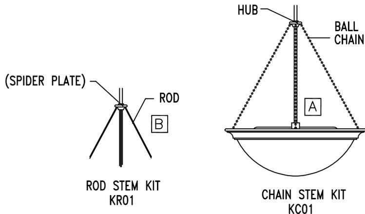
Raise and position spider plate or hub off top of fixture. See chart below for distance.
