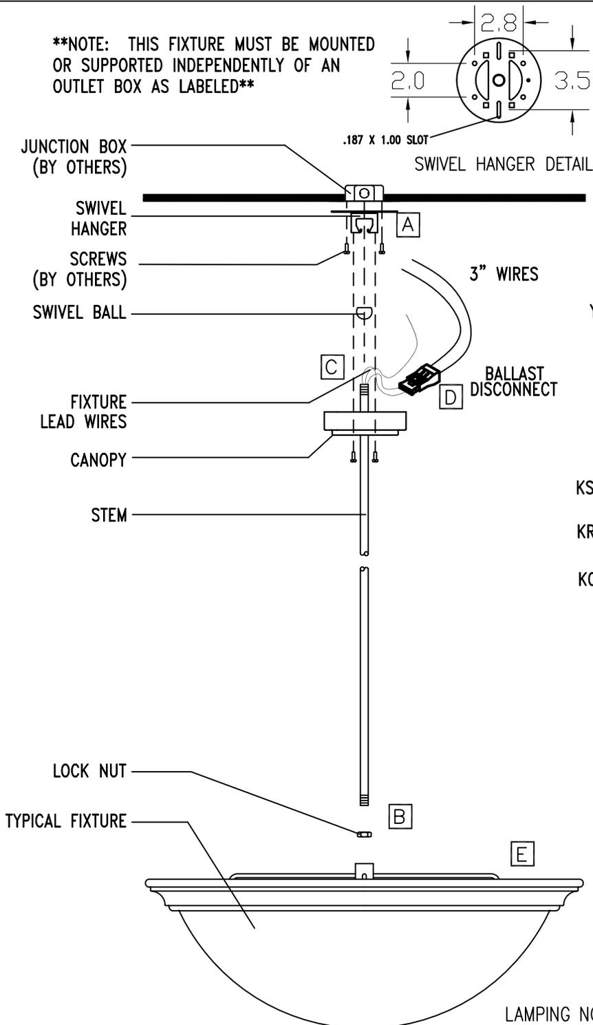
Additional supporting means (by others) for swivel hanger: 1/4" threaded rods to support structure, or 0.88 diameter stem through ceiling to junction box. Fastened with lock nut.
