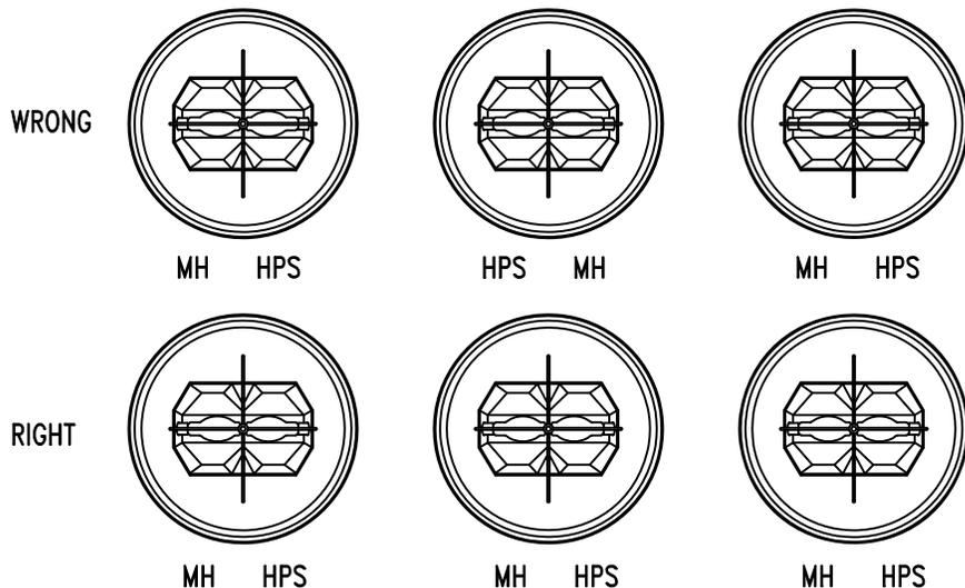
Position fixtures in orientation shown when metal halide and high pressure sodium dual lamp sources are used.
